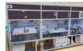
Automated specimen processing device for measuring the quantity of the active ingredient in our ONPO product
